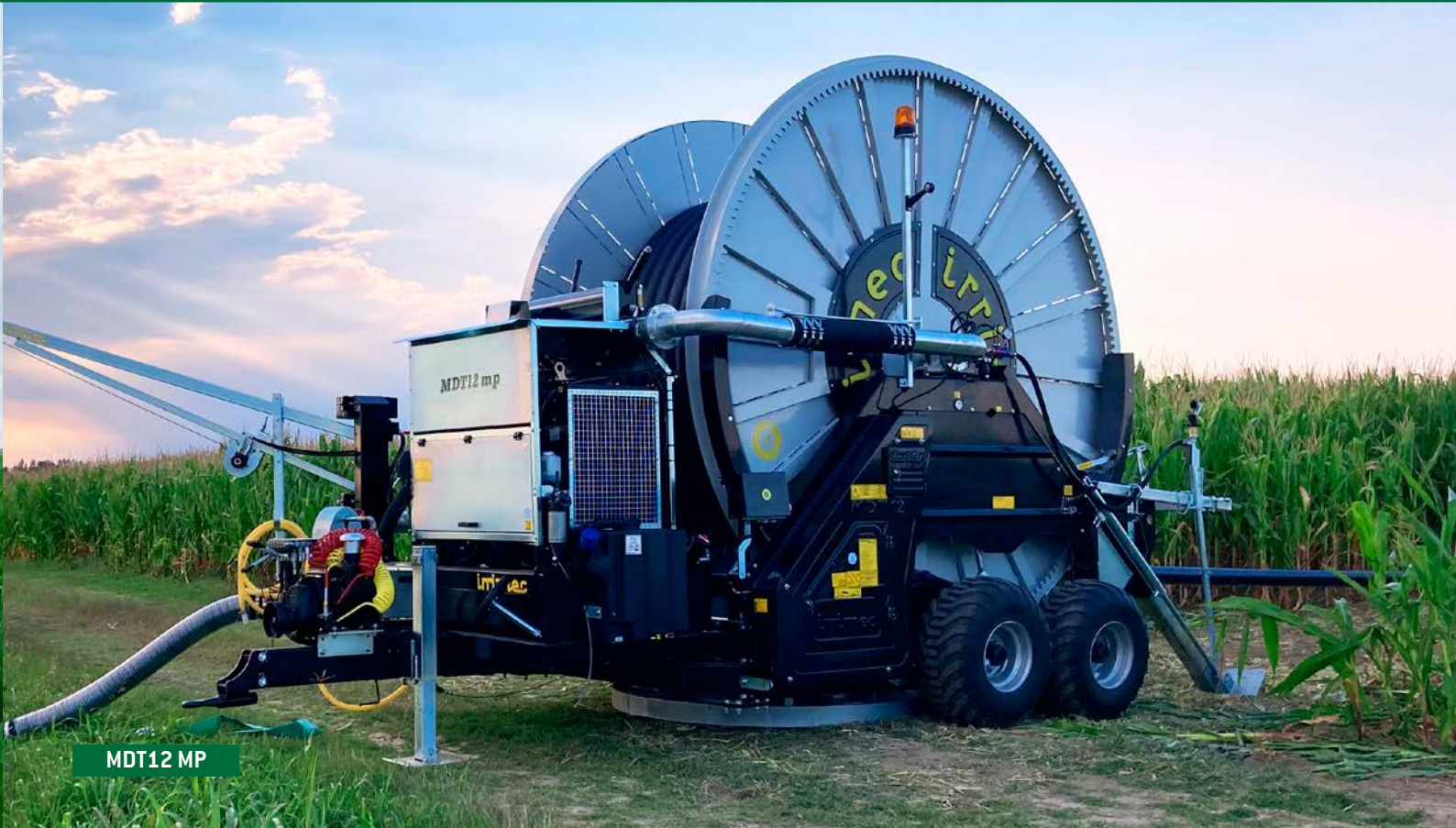
Carrello grossa portata a 4 ruote basculanti Trolley high flow guns with 4 pivot wheels
